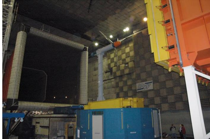
**Figure 3: Set-up of the Mexico model in the LLF tunnel of DNW.**
