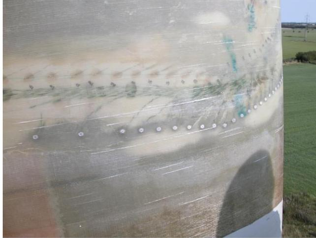
Figure 5: About 50 microphones were installed about one millimeter below the blade surface on the outboard section at radius 37 m for high frequency surface pressure measurements.
