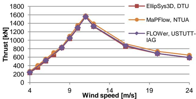
Figure 5: DTU 10 MW thrust curve (modified from [3])
