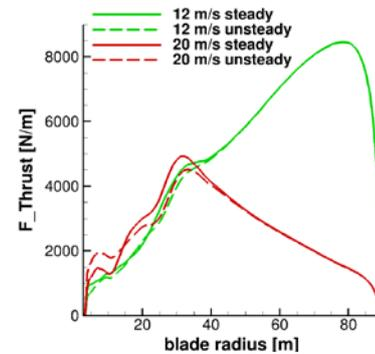
Figure 9: Thrust– comparison steady/unsteady
