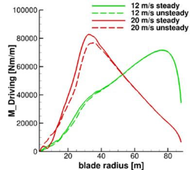
Figure 8: Torque – comparison steady/unsteady
