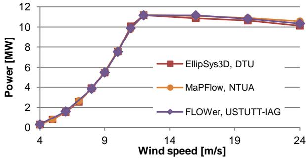
Figure 4: DTU 10 MW power curve (modified from [3])
