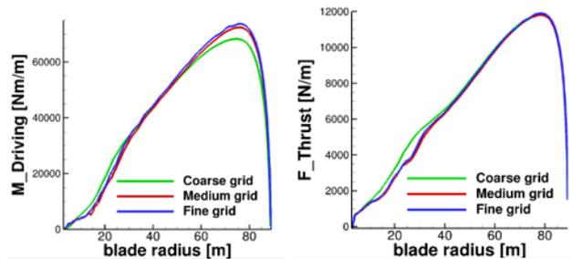
Figure 2: Grid convergence DTU 10 MW turbine
