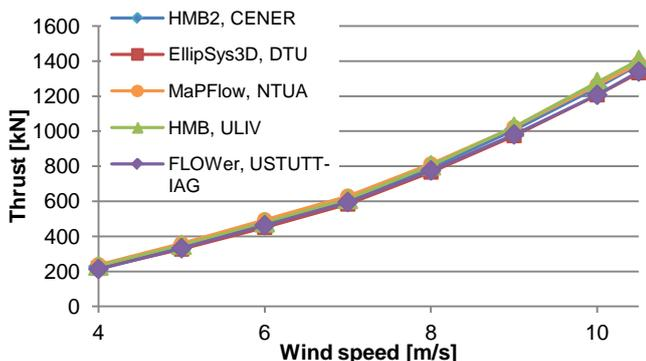
Figure 7: AVATAR thrust curve (modified from [3])
