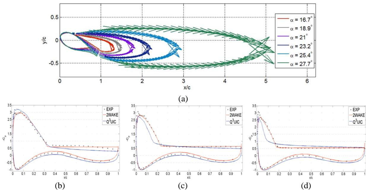
**Figure 3.** (a) Representation of the FFA-W3-301 airfoil and its converged wake shape at different angles of attack ; Pressure distribution around the airfoil in comparison to experimental data and  $Q^3UIC$  at angles of attack (b)  $16.7^\circ$ , (c)  $21^\circ$  and (d)  $27.4^\circ$ .
