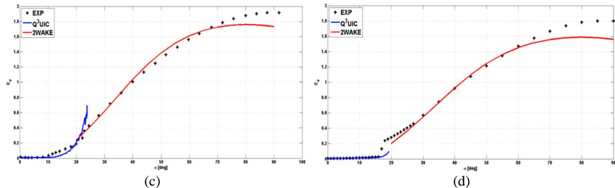
**Figure 8.** Comparison between experimental and computed  $C_l$  (upper) and  $C_d$  (lower) curves at  $Re = 0.7e6$  for (a),(c)DU96-W-180, (b)(d) NACA 0015.
