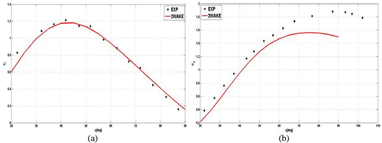
**Figure 6.** Comparison between experimental and double wake simulations for flows past the GA(W)-1 at  $Re = 0.67e6$  (a)  $C_l$ , (b)  $C_d$
